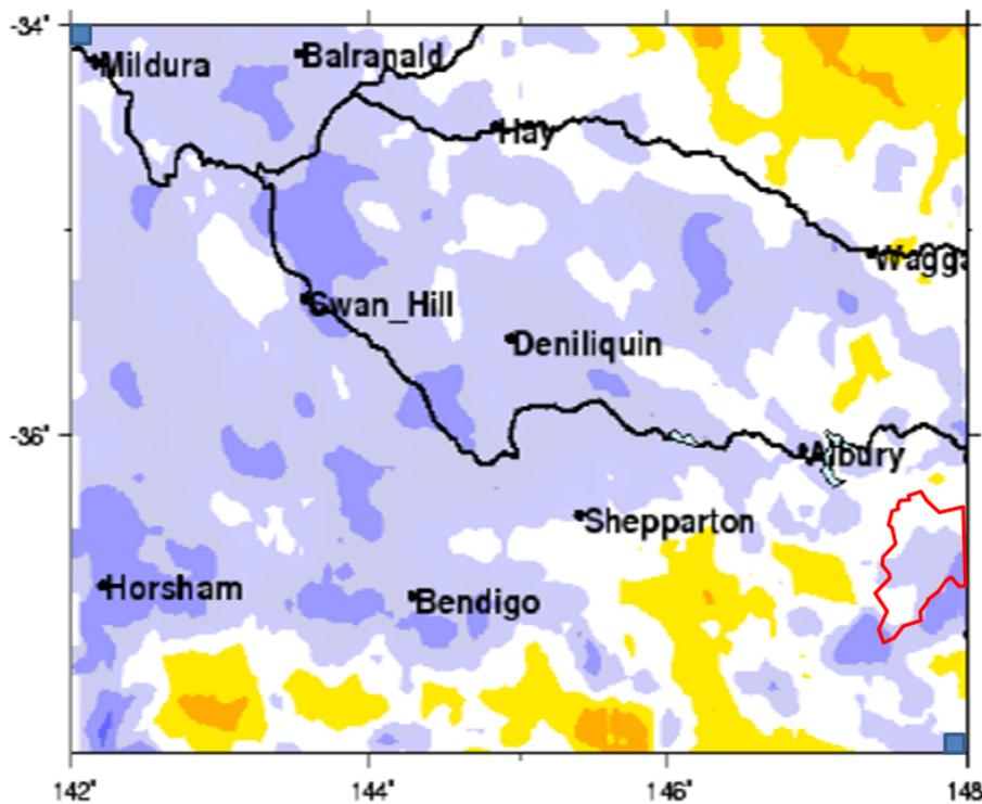
**Figure 2: Projected percentage changes in design rainfall depths for the 24 hr duration under projected 2030 climate conditions, from Abbs (2009), with the Dartmouth Dam catchment area outlined in red.**
