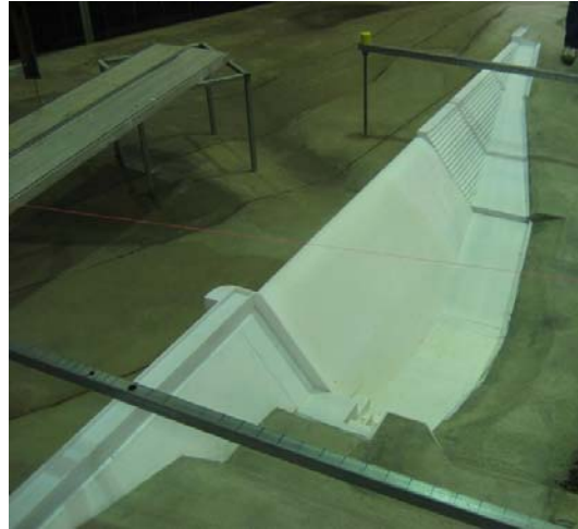
Figure 3 – Wyaralong dam physical hydraulic model
